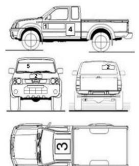
11.4.3 One rally plate must be positioned in a visible position during the whole Rally.It must be fixed at the vehicle, parallel to the axis of the wheels, without covering, even partially, the vehicle's license plate.
